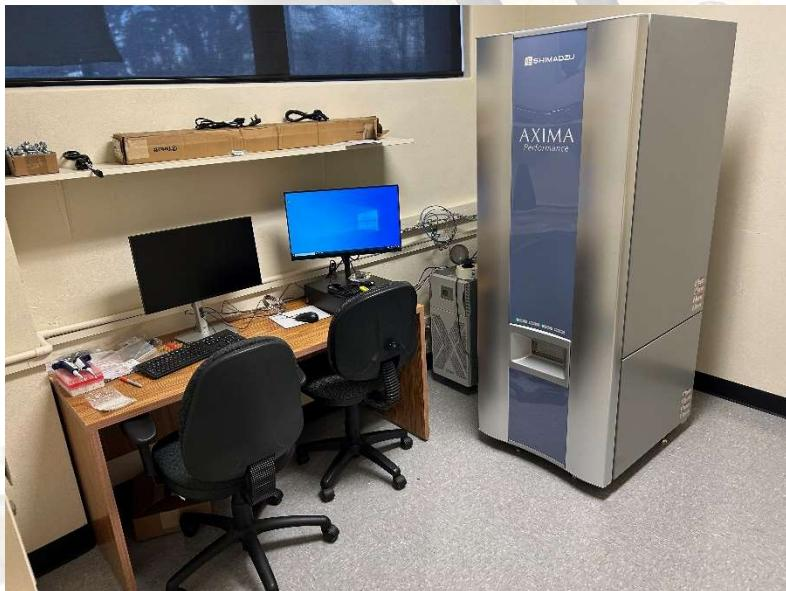
Instrument: Shimadzu Performance MALDI-TOF instrument
